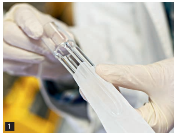
Easy handling: Insert FibreBag, weigh sample and you're ready. No need to seal the filter bag.
